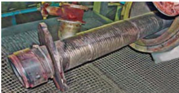
PF-burner lined with KALMETALL®.
