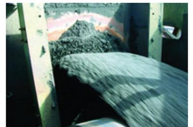
KALIMPACT installed at a ship unloading facility handling taconite.
