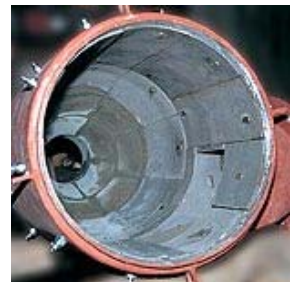
Cyclone used in a soil decontamination system.
