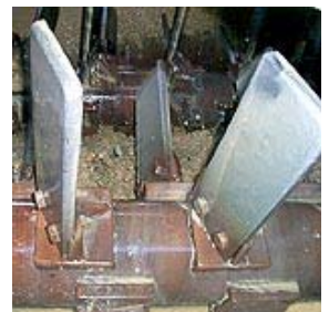
Paddles made of KALCAST® 153 installed in a gravel washing unit.
