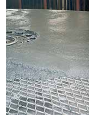
Separators are frequently protected by KALMETALL hard overlay welding or by KALCRET hard compound (pictures) installed without joints.
