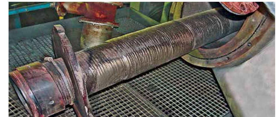
PF-burner lined with KALMETALL.
