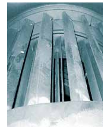
Weight saving design of a separator cage with KALSICA A silicon carbide ceramics; alternative linings are KALMETALL and KALOCER tiles.
