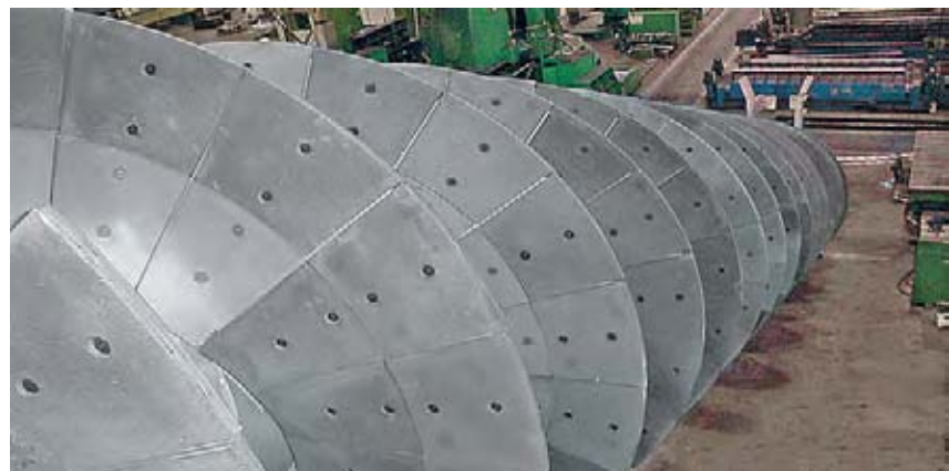
Conveyor screw being part of a slag granulating system; screw flights lined with KALMETALL-C 155; the screw has a diameter of 1,200 mm
