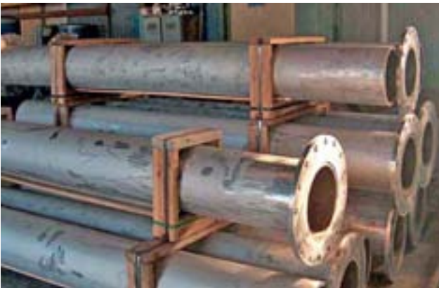
Down pipes of a direct reduction line made of KALMETALL-W 151, 355 mm diameter; basic material 1.4829 of 12.8 mm
