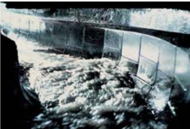
Scale launders are effectively lined with ABRESIST fused cast basalt
