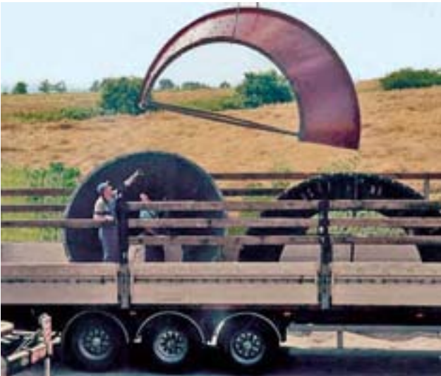
Cyclone separator cones of KALMETALL-W 100 6 + 4 fixed by means of bolt welding
