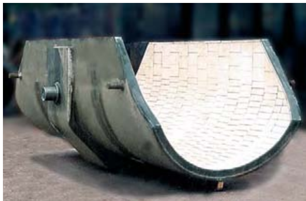
Distributor tilting chute being part of blast furnace lining fitted with KALOCER oxide ceramics, 50 mm thick
