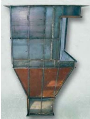
KALCRET hard compound has stood the test as lining material in components of slag granulating systems. Depending on their specific geometry the plant components can be lined within a minimum of time by trowelling or by the spraying technique.
