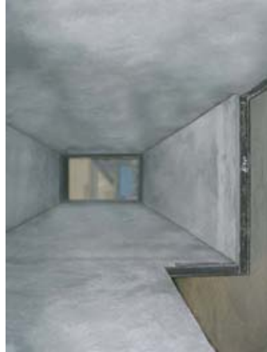
KALCRET hard compound has stood the test as lining material in components of slag granulating systems. Depending on their specific geometry the plant components can be lined within a minimum of time by trowelling or by the spraying technique.
