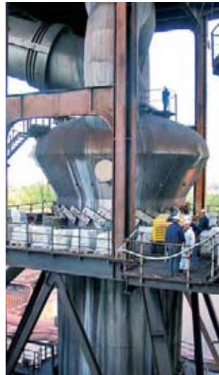
Short lining times for a whirler thanks to sprayed-on KALCRET-BTS hard compound; the high application rate is 5 m 2 /h
