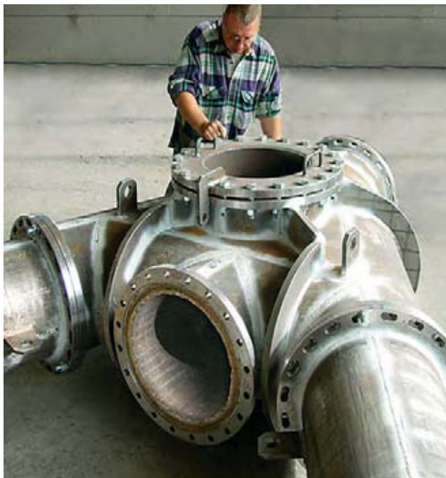
Pressure compensating pipe at the blast furnace; self-supporting structure of KALMETALL-W 100 30 + 6 hard overlay welding; 450 mm Ø
