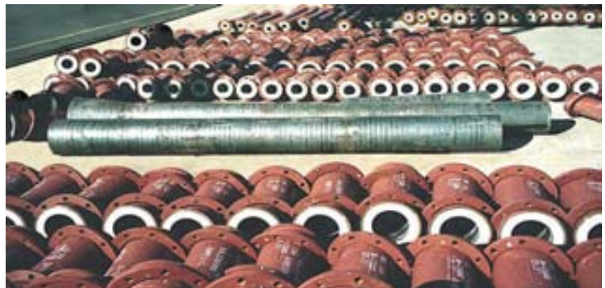
Pulverized coal pipe with ABRESIST and burner tubes made of KALMETALL-W 100; depending on the operating conditions pipes are protected with ABRESIST, KALCOR, KALCRET or KALOCER
