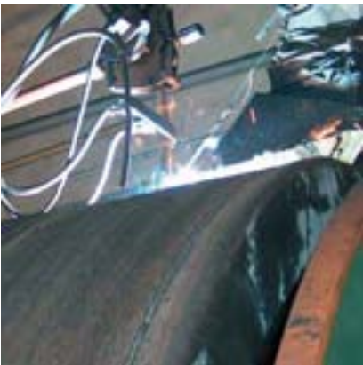
Service by Kalenborn: rebuilding of a grinding roll with KALMETALL-W 100
