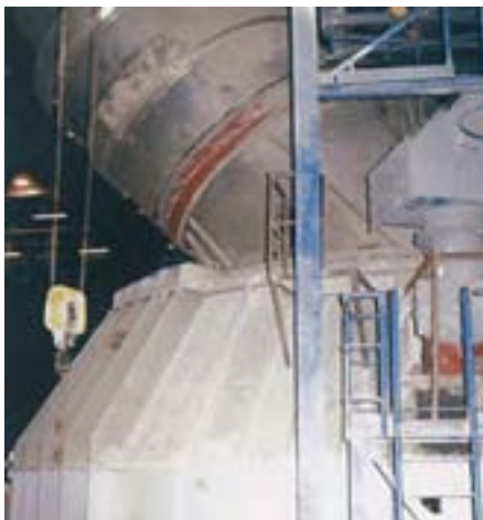
Housing made of KALMETAL-W for a raw meal fan – 2,000 mm Ø – as self-supporting structure
