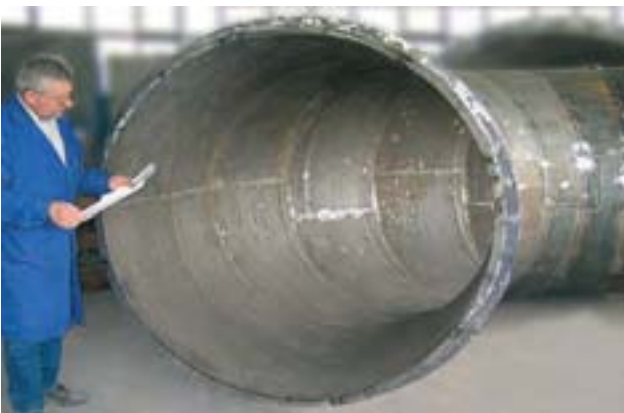
Clinker dust pipe: cyclone exit protected with KALMETALL-W
