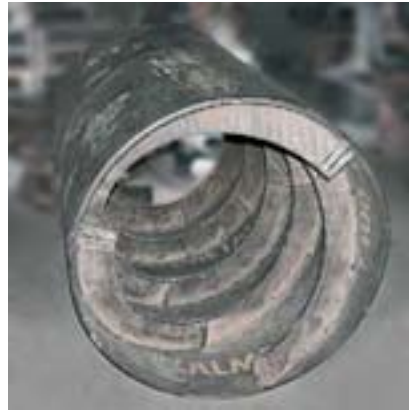
Conveyor for clinker transport lined with KALMETALL-W 100; 800 mm Ø
