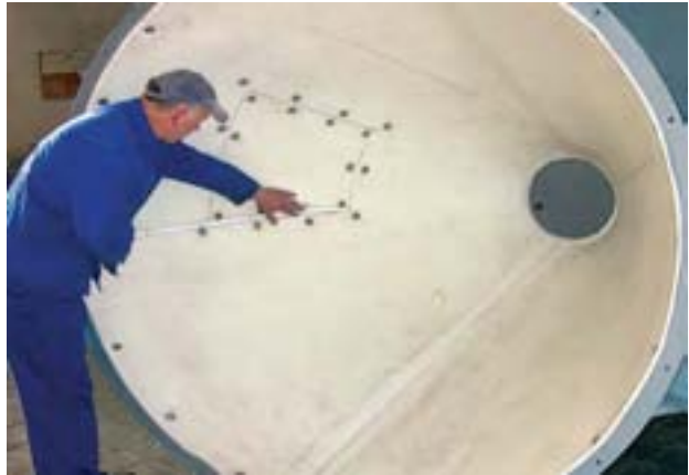
KALOCER high alumina ceramics lining of a separator with mechanically fixed tiles, 100 x 100 mm
