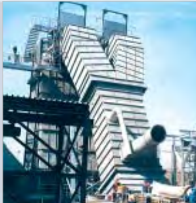
Lining of a cooler pipe that handles clinker in a cement plant with KALCRET-BNY hard compound; the prefabricated shaped elements with integrated insulation have been provided with mechanical fastening system
