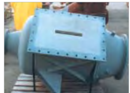
Hot gas cyclone designed for temperatures of 1000 °C / 1832 °F
