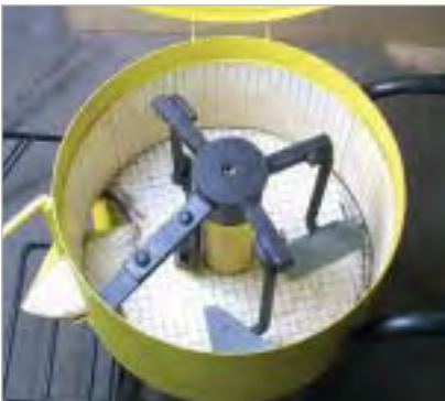
Wear protected tank of a KALCRET forced circulation mixer
