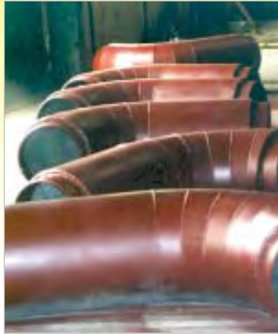
Pulverized coal bends for a power plant with prefabricated KALCRET pipe bends
