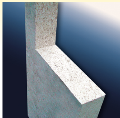
The cut surface indicates the dense, homogenous structure of KALCOR-S. The surfaces are practically free of voids.
