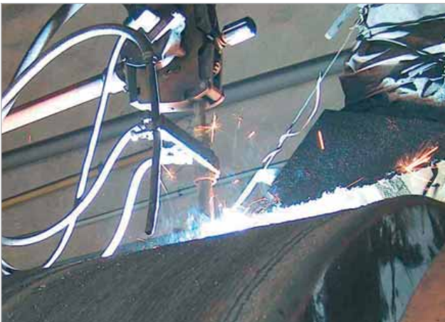
Regeneration of grinding rolls is a time-tested standard of the Kalenborn welding service
