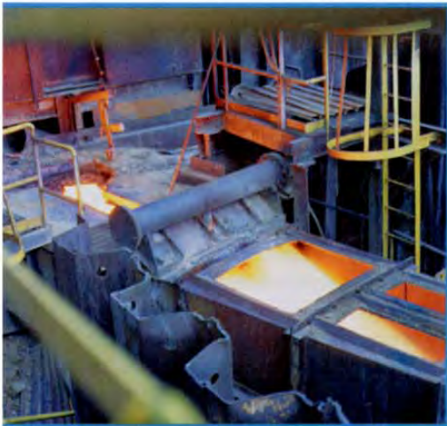
Molten slag flows from the "L" blast furnace at the rate of 3 to 10 tons per minute. Depending on the condition of the molten slag, it will be channeled to a pit for air-cooling or is granulated.
