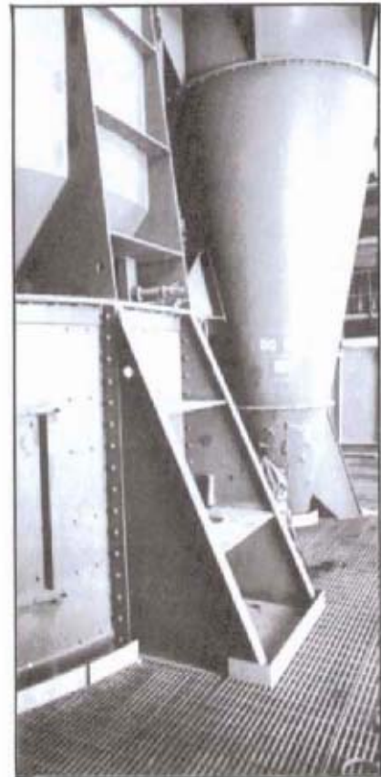
A portion of the air separator, flanked by two of its four cyclones. The system handles 390 st/h during "steady state" operations, achieved 1½ hours into an operating cycle—140-145 st end as finished product, while 250 st/h are recycled to be fed through again.
